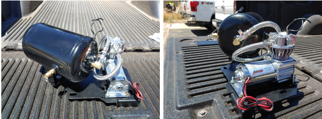
Figure 15- Compressor Hose Routing (Recommended)
