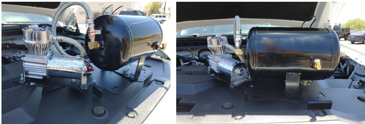
Figure 19- Compressor Hose Routing (Recommended)
