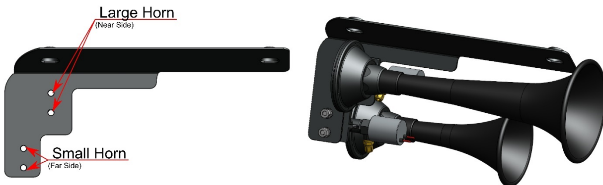
Figure 24- Horn Installation, 2015 to 2020 SUV's
