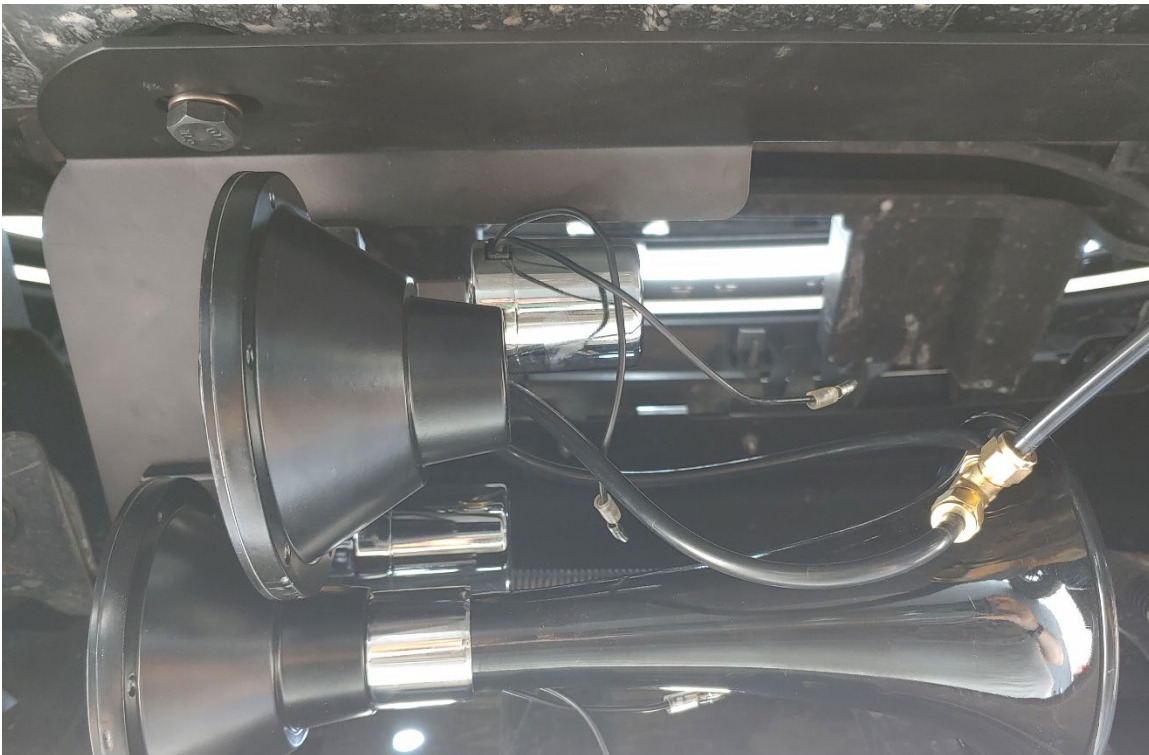
Figure 33- Horn Bracket Installed, Upper Trumpet Removed (Shown)
