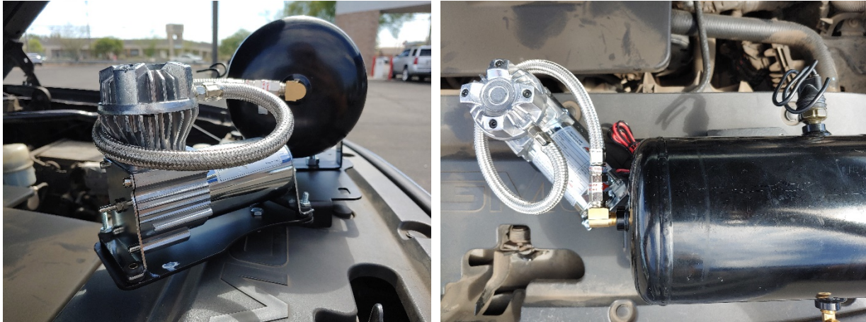
Figure 23- Compressor Hose Routing (Recommended)
