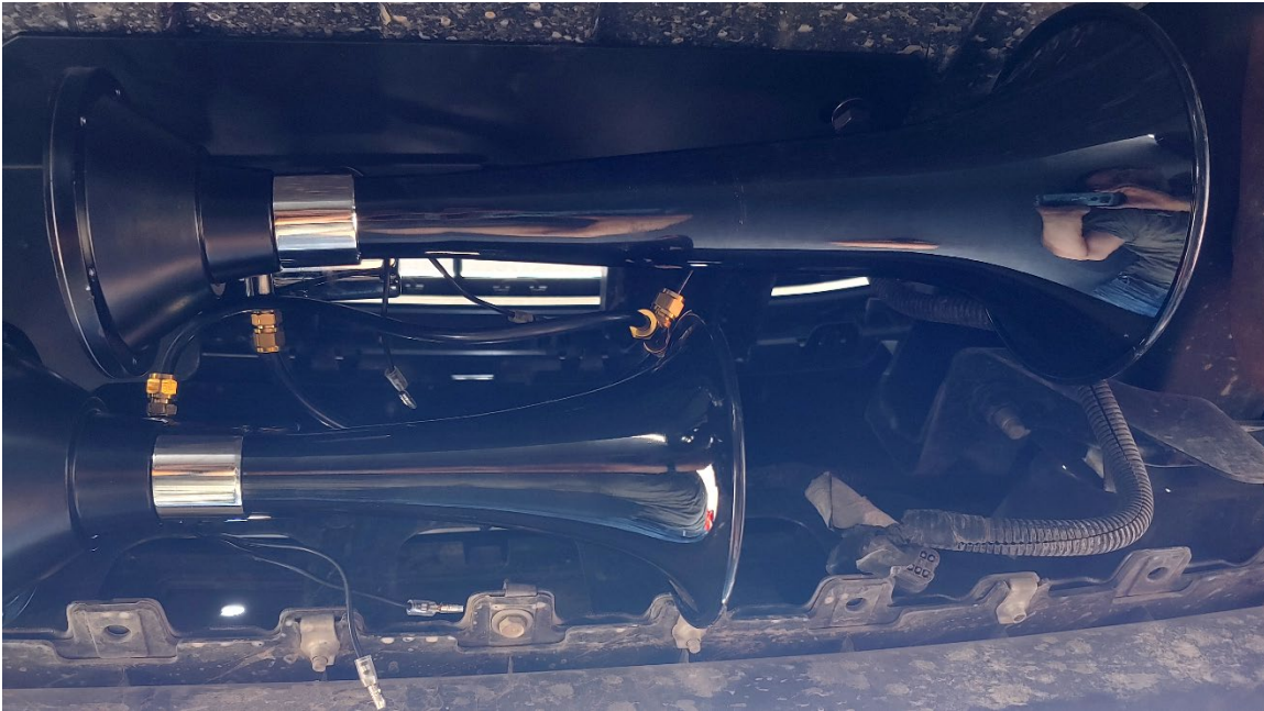
Figure 31- Horn Bracket Installed Location, Behind Front Bumper
